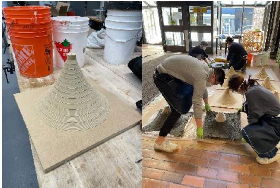
Fig. 5. An assembled MDF conical mold (left), and a concrete cast towel being cast onto the mold (right)
